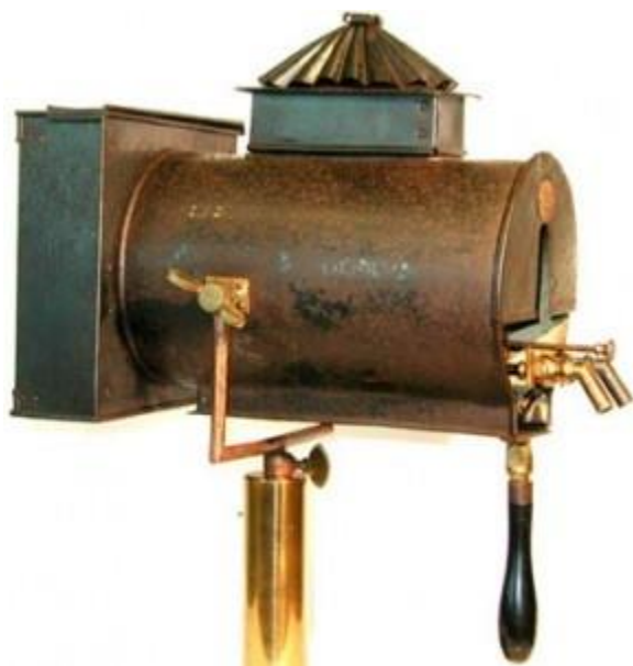
Fig. 35, A gas limelight powers this spotlight / work light.
