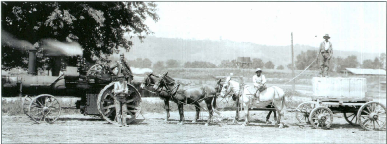
An O. S. Kelly traction engine assisted a mule team to move a 3,600-pound Bedford limestone block to River Station after a heavy rain. Between 1890 and 1891, Oliver Kelly employed designing engineer Edward T. Wright, an Englishman who apprenticed at Aveling & Porter. Wright's influence may be detected in the design of the Kelly engine.
