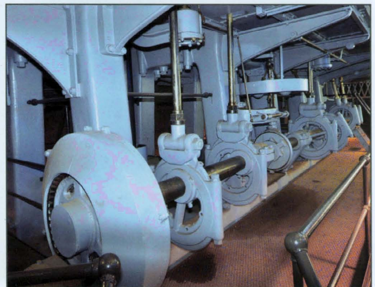
Hook rods from the valving deck attach to the eccentric bearings on a 30-foot shaft.
