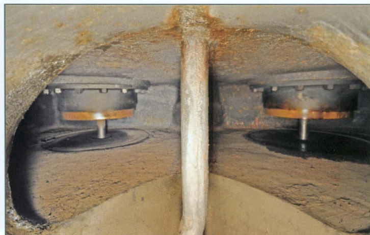
Shown is the steam chest view of the 14-inch balanced poppet valves for the crank end on the exhaust side of the low pressure cylinder.
