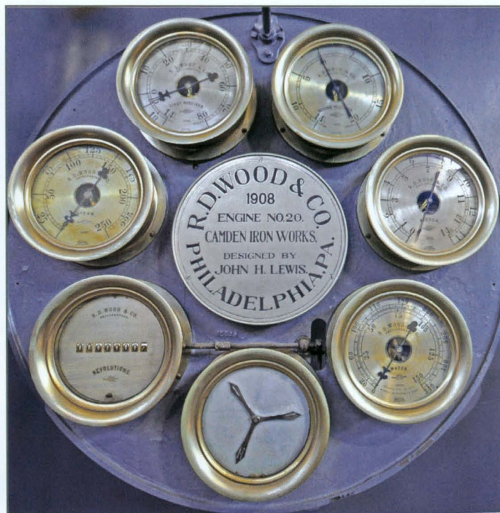
The bottom dial on the gauge panel is a CCW rotating piston position indicator (PPI), displaying the real time location for all three steam pistons and pump plungers. The starting procedure changed in response to the location of the piston in the high pressure cylinder.
