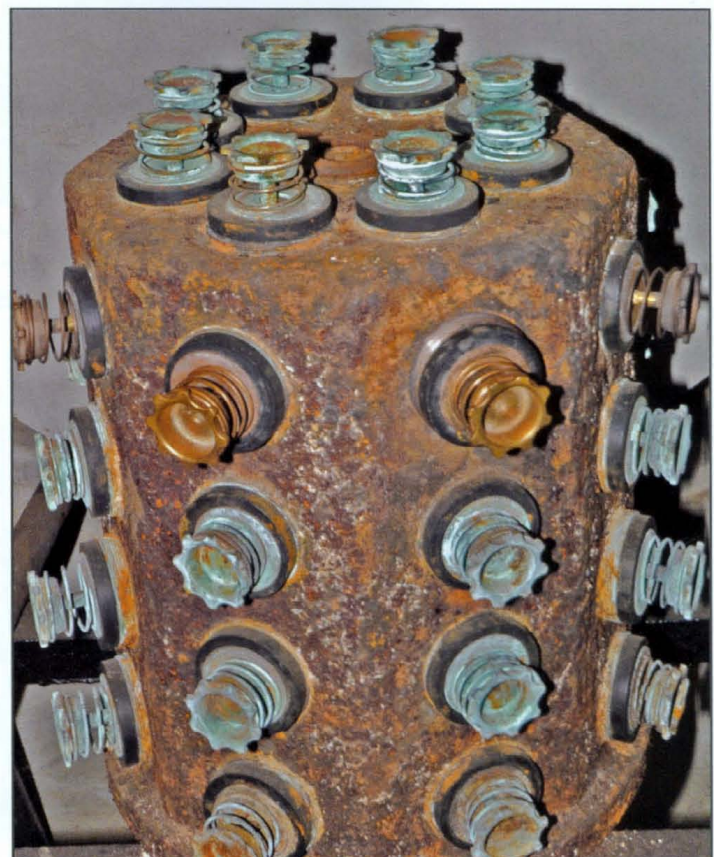
Removed from the engine for display purposes is one of 14 poppet valve cages in each pump.
