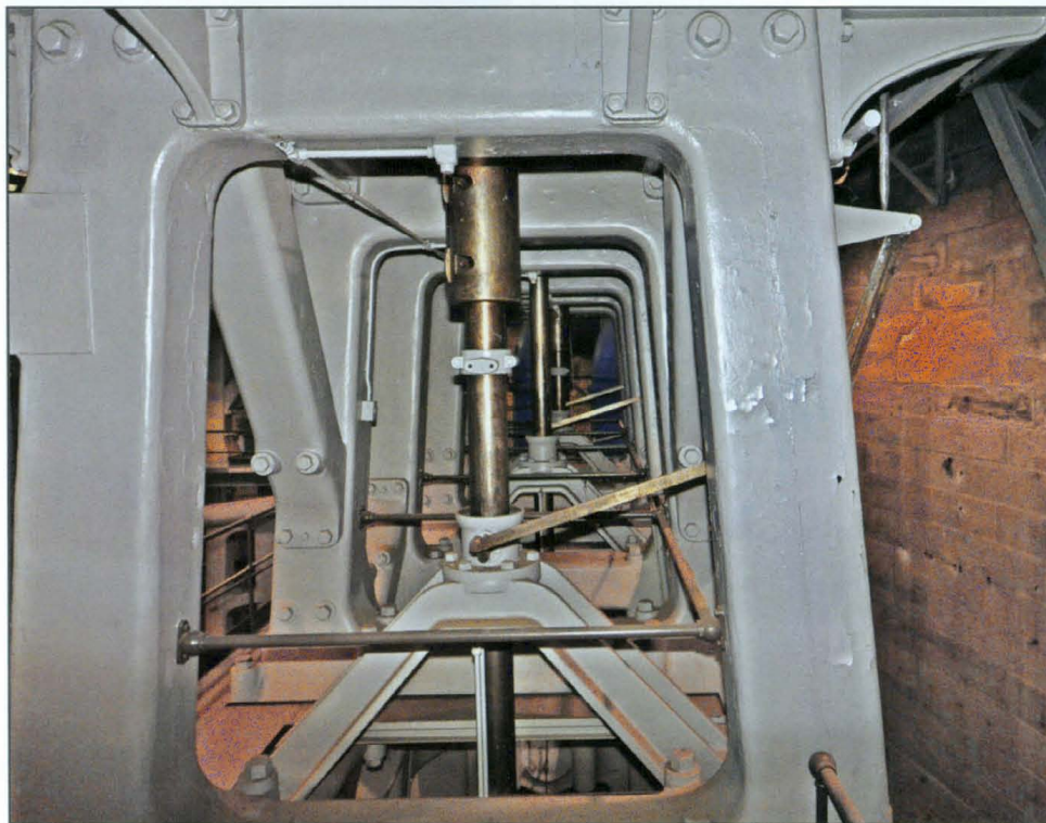
Levers to power all three steam indicators are normally attached to the connecting rods, but here they are shown in their resting position on the housing for the stabilization bearings. They extend upward to the operating deck at the rear of the engine.
