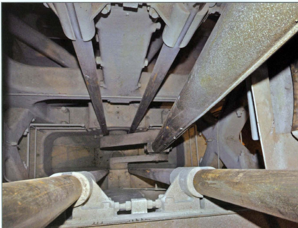
The quad connecting rods from the crosshead to the pump plunger straddle the crankshaft and the crank web.
