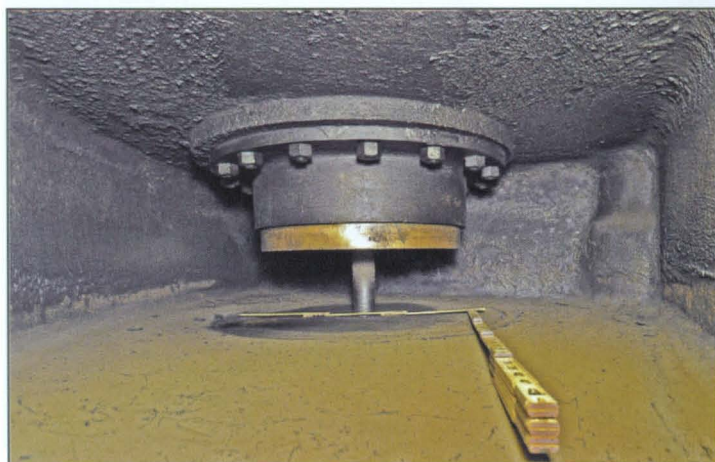
Pictured is one of two balanced poppet valves in the steam chest for the crank end on the exhaust side of the low pressure cylinder.
