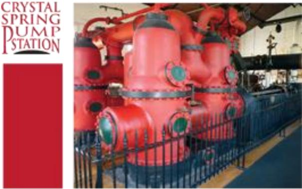
Snow Horizontial Compound Water Pumping Steam Engine
